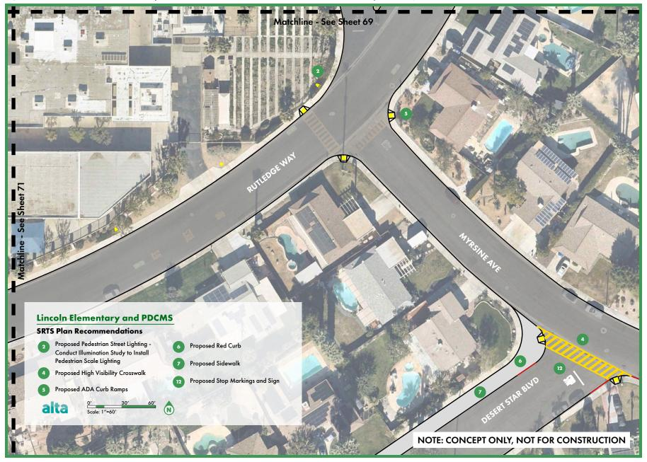
**Lincoln Elementary and PDCMS SRTS Plan Recommendations** Proposed Pedestrian Street Lighting -Conduct Illumination Study to Install Pedestrian Scale Lighting See Sheet 72 **RUTLEDGE WAY** NOTE: CONCEPT ONLY, NOT FOR CONSTRUCTION
