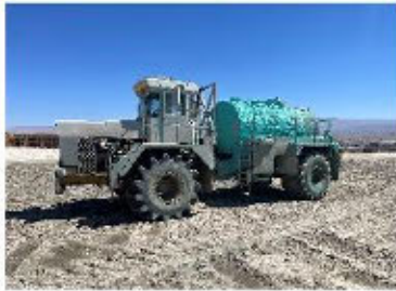
Chemical Dust Suppressant (CDS) Application: Soil binder is routinely applied to inactive or high sensitivity areas to control dust emissions. See attached records.
