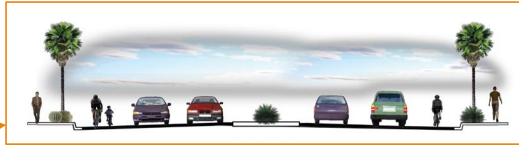
BALANCED ARTERIAL (4 LANES, DIVIDED) WITH BICYCLE LANES
