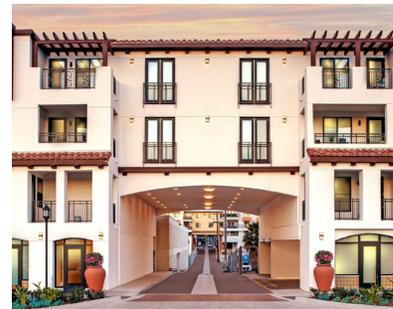
▲ Vehicles entering this multifamily building can queue in the covered passageway and turn right into the garage, avoiding blocking the sidewalk. See ODS 5.4.2.
