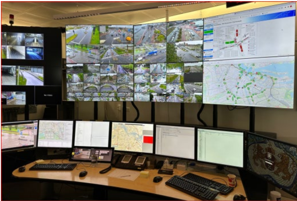
Amsterdam’s Traffic Operations Center – Note four screens visualize free (e.g., Google Maps) public-sourced traffic data blended with surveillance cameras and municipal traffic signal data. (photo by Dave Zelenok, September 2023)
